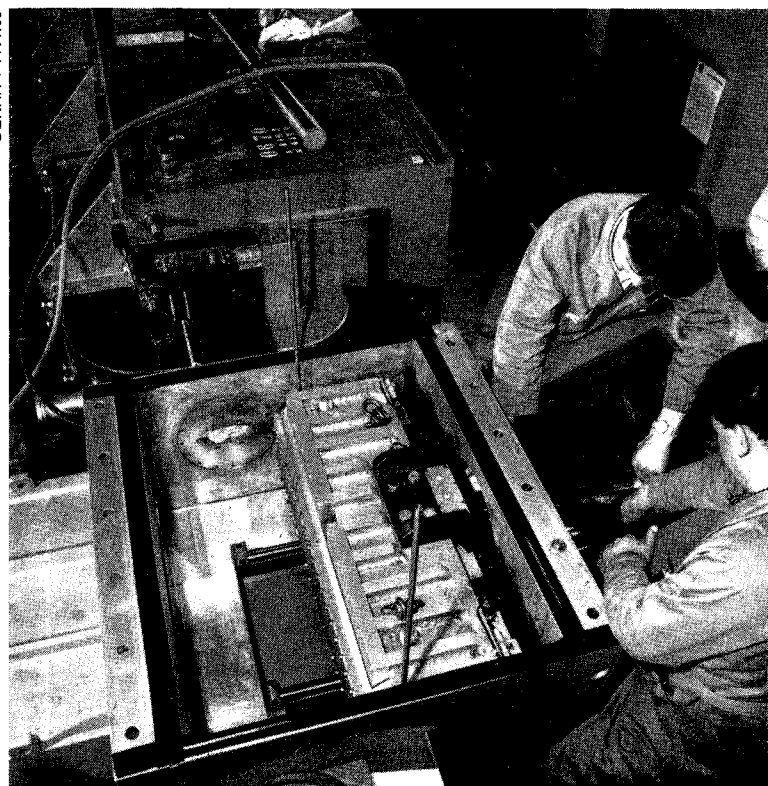
3. The kicker magnet FK 97 installed in its vacuum tank in straight-section 97 of the synchrotron. The tank cover is off and the magnet can be seen in its withdrawn position out of the beam path.
